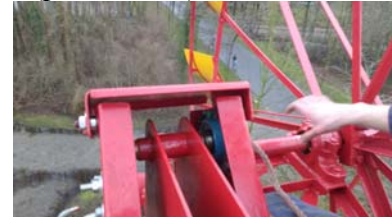
rotor and main shaft (massive Ø 50h6 C45) (photo 2017)
