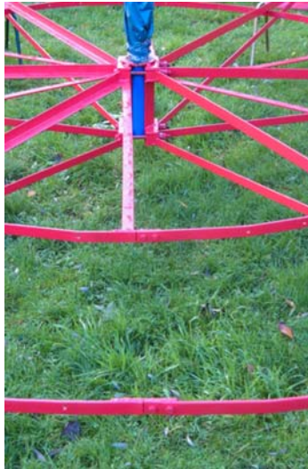
main shaft, clamp, two rotor-halves assembled (photo 2005)
