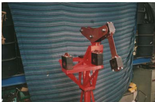
head, tumbler, conrod, wooden bearings (photo 1993)
