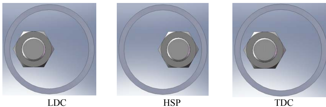
Fig. 5.4: pumprod (Ø16mm) with hexagon nut in rising main (2" gaspipe), top view
