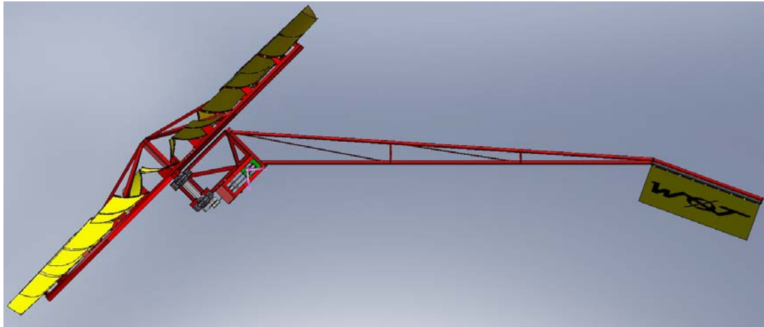
modest windspeeds, vane almost vertical (top view)
