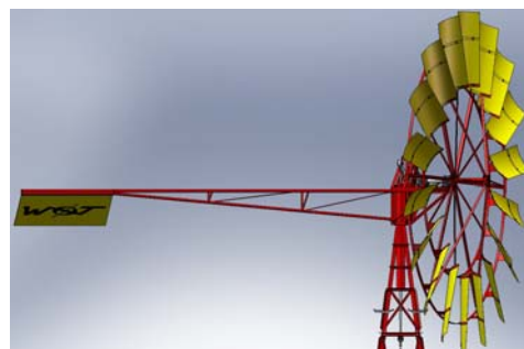
high windspeeds: rotor approx. 70° out of the wind vane almost horizontal
