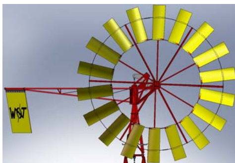
modest windspeeds: rotor approx. 8° out of the wind vane almost vertical
