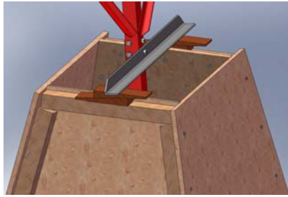
welded tower with anchor
