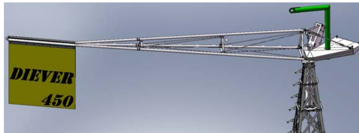
Fig. 6.8: fitting of tail: hoist sling at arrow, chain hoist on jib (shown in green), the top-pipe of tail (axis of vane hinge) must be set horizontal (with turnbuckle M16). tighten the bolts which function as hinges (2 x M16) and the counter nut on turnbuckle (tightening torque: 230Nm)
