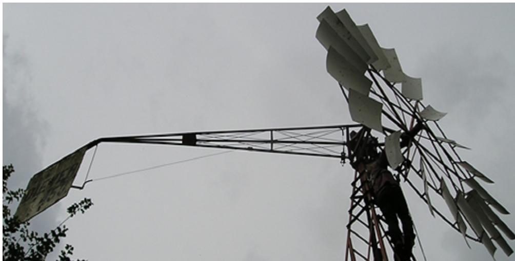
Fig. 6.5: vane hinge: 2½" gaspipe, rubber sheet, vane locking device (photo 2004)
