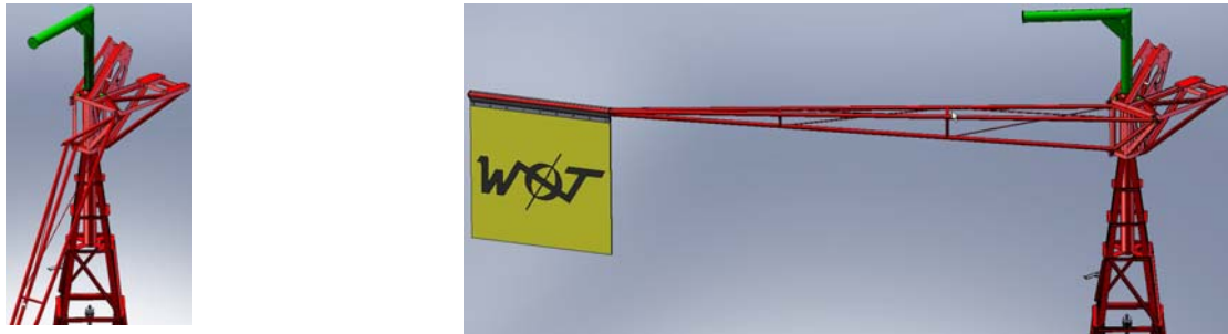
Fig. 6.4: fitting of tail: hoist sling at arrow, chain hoist on jib (shown in green), the two top-pipes of tail (axis of vane hinge) should be horizontal when the bolts (6 x M12) have been tightened (tightening torque: 90Nm)
