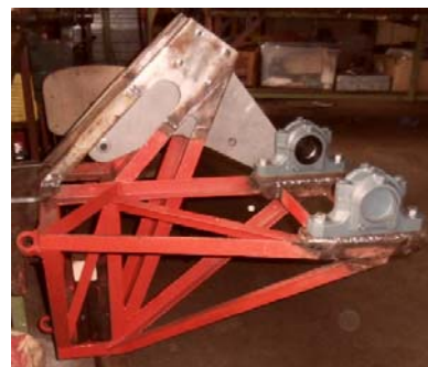
head, tumbler, rolling bearings (photo 2016)
