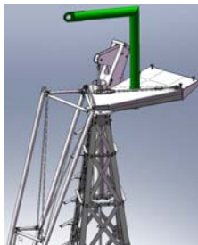
Fig. 6.8: fitting of tail: hoist sling at arrow, chain hoist on jib (shown in green), the top-pipe of tail (axis of vane hinge) must be set horizontal (with turnbuckle M16). tighten the bolts which function as hinges (2 x M16) and the counter nut on turnbuckle (tightening torque: 230Nm)
