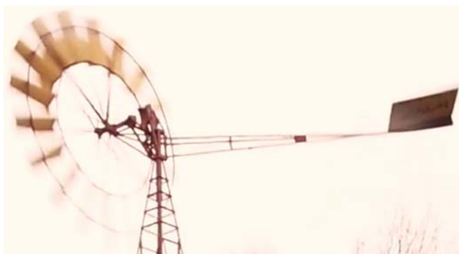
Fig. 9.1: behaviour Diever 450 at storm conditions: windforce 9, windgusts of 33m/s at testfield (snapshot of film made 18 January 2018)
