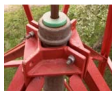
Fig. 11.3: pumprod guide and clamp for rising main (photo 2018)
