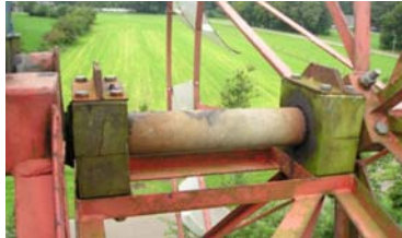
rotor and main shaft (gaspipe 2½") (photo 2004)
