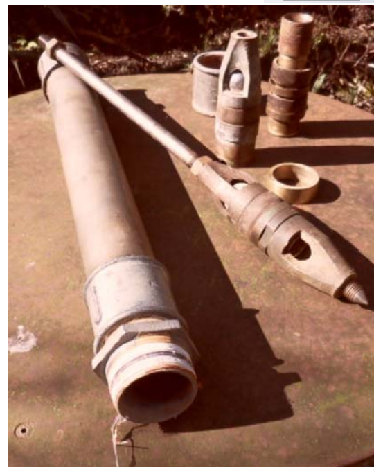
extractable pump (E) (photo 2018)
